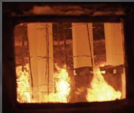
Columns exposed to a standard ASTM E119 (UL263) fire exposure
