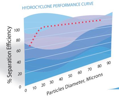
ERMA FIRST BWTS, through the innovative hydrocyclones, which allow particles of only less than 10 microns to enter the Ballast Tanks, is the only Ballast Water Treatment system that provides THE MOST CLEAN SEA WATER to both the ballast tanks and to the disinfection unit, thus further eliminating re-growth, reducing sediment amount in the BW tanks (further minimizing maintenance costs in Drydock) and reducing energy consumption of the disinfectant unit (i.e. electrolysis cells).
